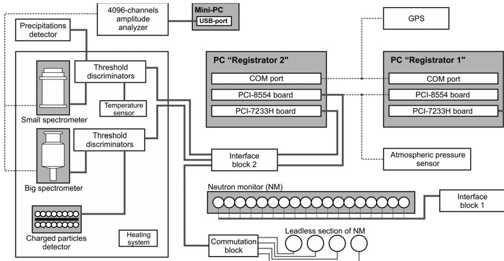
Figure 1: The functional diagram of the complex set for cosmic rays monitoring in Apatity. The small spectrometer has  $\text{Ø}60 \times 20$  mm NaI(Tl) crystal, the big one has  $\text{Ø}150 \times 110$  mm. Due to the amplitude analyzer the big crystal is used for measuring of the differential energetic spectrum of gamma-rays.
