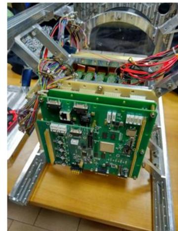
Fig.1. Left panel: The Mini-EUSO instrument 3D model. Right panel: the PDM-DP boards in the Mini-EUSO engineering model during tests.
